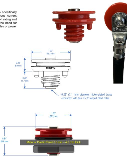
For complete dimensions, download 3D Step files of Terminal and Accessories at Rebling.com
