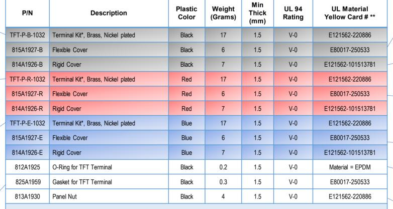
\*Terminal Kit = one Terminal + one Panel Nut + two Bolts + two Split Washers, all parts in a small poly bag \*\*UL Material Yellow Cards can be downloaded from ULprospector.com
